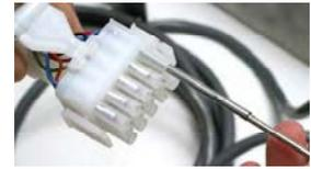
**DO** use a pin pusher to remove the 15-pin plug on the controller cable for routing.
